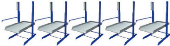
Without post sharing, 5 units need 10 posts
