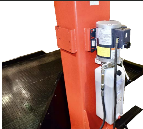
Three Power unit mounting brackets - front & sides of column
