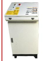
220V 1PH 60 HZ **POWER UNIT** 3HP MOTOR 30 AMPS 120 PSI AIR SUPPLY 115 SECS RISE TIME
