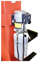
THREE POWER UNIT MOUNTING BRACKETS - FRONT & SIDES OF COLUMN
