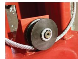
3/8" / 9.5MM CABLES - 4 3/8" / 111MM PULLEYS
